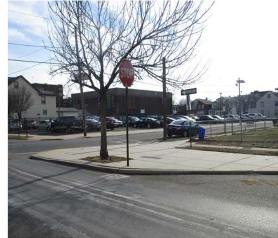
Stormwater is currently draining to nearby catch basins. Tree filter boxes can be constructed along the eastern sidewalk to capture and treat stormwater runoff and provide additional landscape value to the site. A preliminary soil assessment suggests that more soil testing would be required before determining the soil's suitability for green infrastructure.
