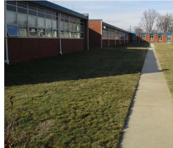
Stormwater is currently draining across the site to nearby catch basins. Building downspouts can be disconnected and directed into rain gardens. Installing rain gardens adjacent to the building can capture, treat, and infiltrate roof runoff. A preliminary soil assessment suggests that more soil testing would be required before determining the soil's suitability for green infrastructure.
