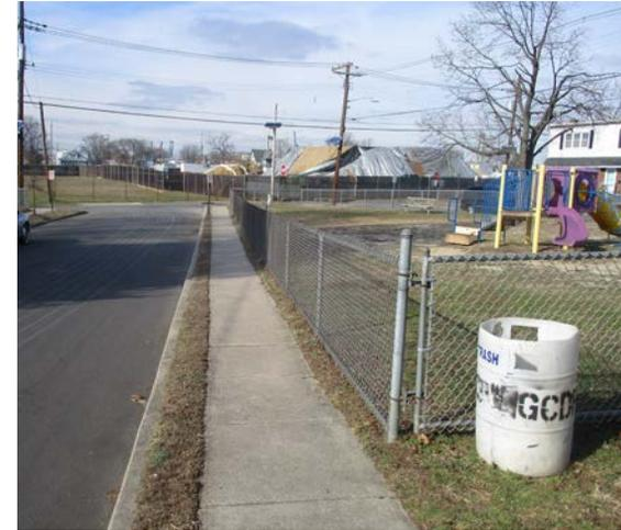
Stormwater is currently draining from south to north across the site. Tree filter boxes can be constructed along the northern sidewalk to capture and treat stormwater runoff and provide additional landscape value to the site. Adjacent sidewalks can be converted to porous asphalt to capture and treat stormwater runoff. A preliminary soil assessment suggests that more soil testing would be required before determining the soil's suitability for green infrastructure.
