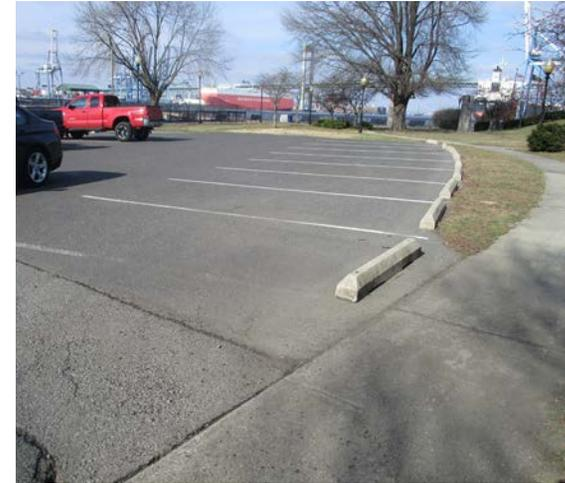
Stormwater is currently draining from east to west across the site. Parking spaces in the Proprietors Park parking lot can be converted to porous asphalt to capture and treat stormwater runoff. Stormwater can be diverted from the road into a rain garden. Installing a rain garden adjacent to the roadway can capture, treat, and infiltrate runoff. A preliminary soil assessment suggests that more soil testing would be required before determining the soil's suitability for green infrastructure.
