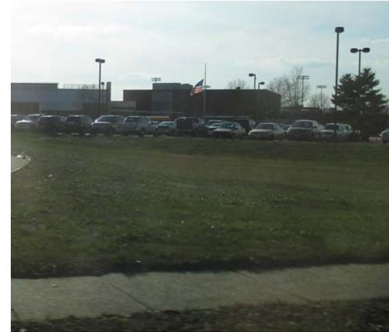
Stormwater is currently draining across the site into a nearby field. The grassy area north of the parking lot can be converted into a rain garden. Installing a rain garden adjacent to the parking lot can capture, treat, and infiltrate stormwater runoff. A preliminary soil assessment suggests that more soil testing would be required before determining the soil's suitability for green infrastructure.
